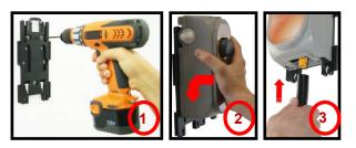
**STEP 1:** Use the backplate as a template to mark the mounting hole pattern. Drill a hole for the supplied ¼" anchors and mount the bracket with the screws provided in the accessory kit.
